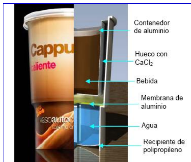
Figure 6. Diagram made by first-year undergraduate students of a self-heating beverage container. Own elaboration based on a drawing made by the author's students.
